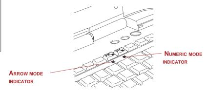
Figure 2-8 Keypad overlay indicators
